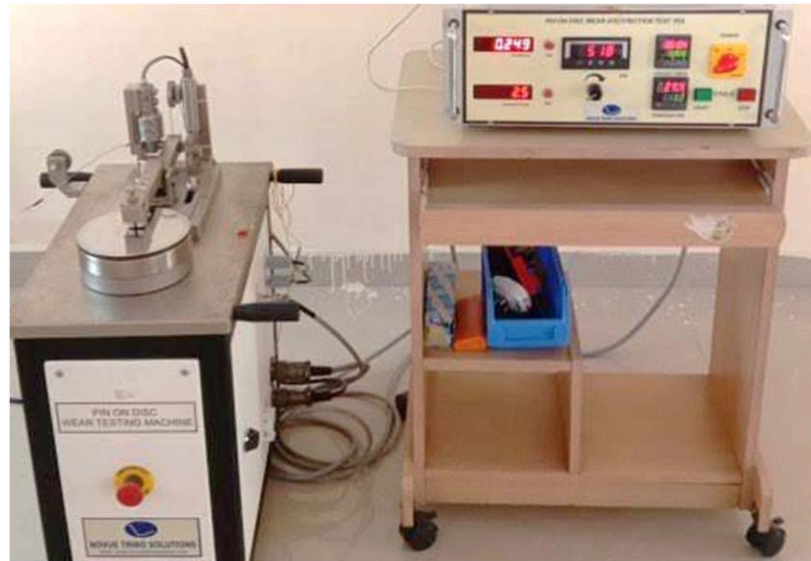
Figure 3. Wear testing set up—Pin on disc apparatus.
